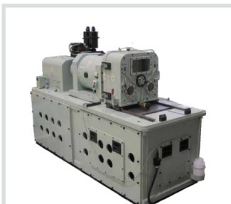
BPH-321-31 • For trucks (MT) • 4000rpm • \pm 3.5\text{kN}\cdot\text{m} \pm 50^\circ • With chamber
