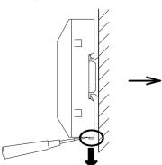
Insert a flathead screwdriver into into the hole of the fixture at the bottom of the main unit and move the fixture downward.
