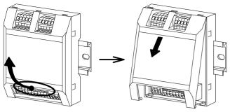
Place your fingers at the bottom of the cover and lift it in the direction of the arrow.
