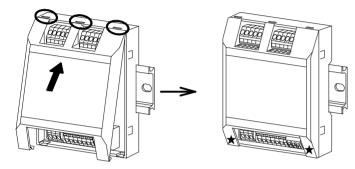
Insert the claws at the top of the cover into the grooves (3 places) at the top of the main unit.
